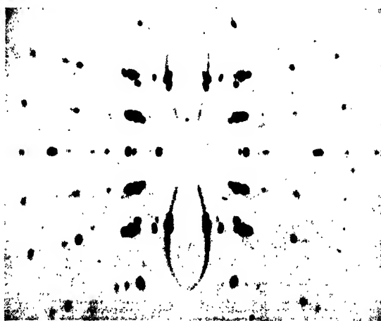
FIG. 4.—Rotation photograph of a monoclinic crystal of diphenyl about the [100] axis. Unfiltered copper radiation. Flat photographic plate.
